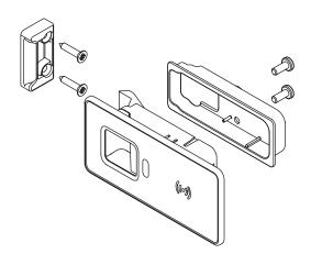
Scope of delivery 2: for mounting with center stop
